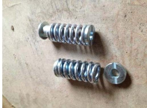
4) Assemble these 2 springs into the hinge, you need to have the 2 legs of pressing pieces go into the notches of the sliding pieces that attached into Springs.
