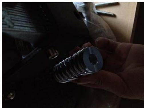
5) Assemble the 2 springs into the hinge, you may need the special tool(Wood Piece or Bamboo Piece) to get the 2 springs into the hinge.
