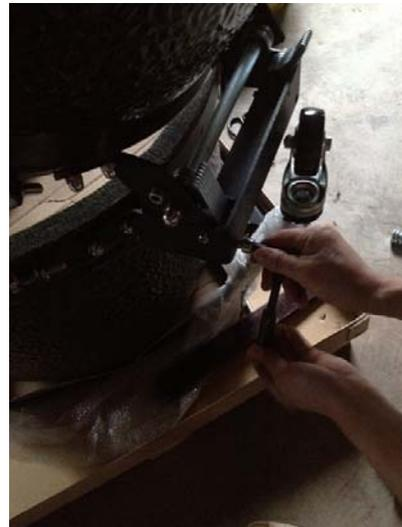
**Warning: do not try to tighten the 2 long big bolts enough when the ceramic dome is open, just tighten loosely.**
